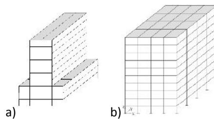
Figure 1. The 3D view of the case study building a) setback structure status, b) regular structure status
