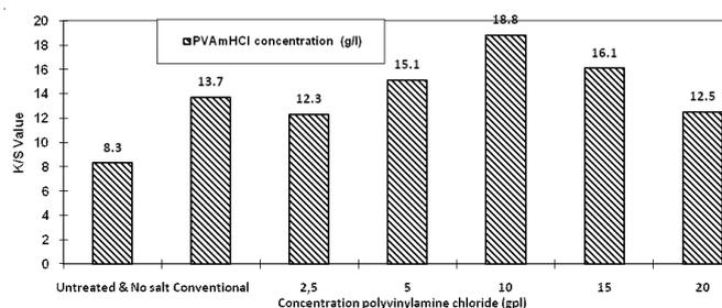
**Figure 1.** K/S value of control and treated samples.
