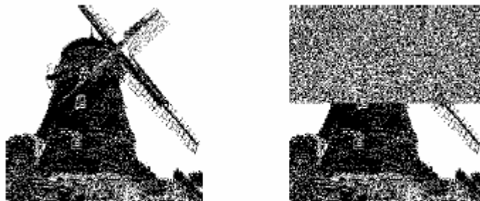
Fig. 3 Least significant bits of pixels (after ordering the palette), it is easy to recognize that there was a hidden message embedded in the right picture.
