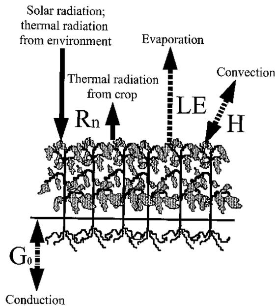
Fig. 1. Simplified schematic diagram of a surface energy balance for a crop with a uniform, closed canopy. Arrows denote direction of energy transfer.  $R_n$  = net radiation;  $G_0$  = soil surface heat flux (conduction);  $H$  = sensible heat flux (convection); and  $LE$  = latent heat flux (evaporation).
