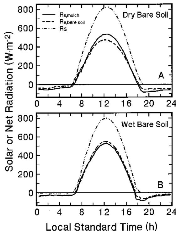
Fig. 7. Net radiation ( $R_n$ ) and total solar radiation ( $R_s$ ) for black plastic mulch and bare soil near Manhattan, Kans., on Day of Year 248 (dry, bare soil) and 272 (wet, bare soil), 1996.  $R_s$  was measured by a pyranometer (Model 8-48; Eppley Laboratories, Newport, R.I.) mounted 2 m above the field.  $R_n$  was measured as in Fig. 4.
