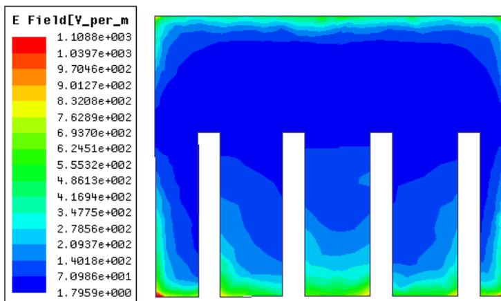
Fig. 5. Current distribution at 1.35GHz
