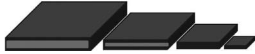
Figure 1. Conceptual view of the distribution of the internal surface area for four different particle sizes. The black part represents the disturbed zone and the grey part represents the undisturbed volume. The smallest particles consist entirely of disturbed zone.
