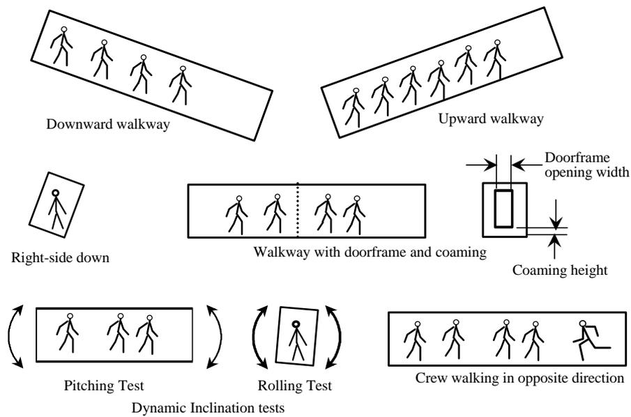
**Figure-7 Test conditions on inclined walkways**
