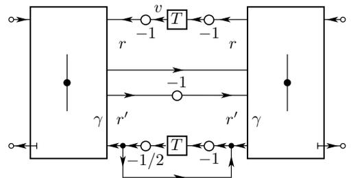
Figure 5: Wave digital structure for the passive 2-stage TSRK method.
