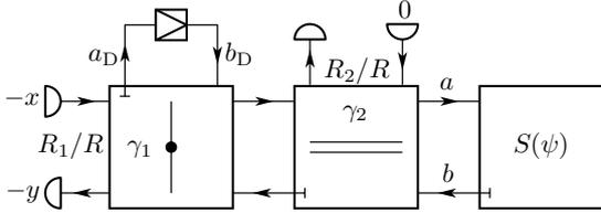
Figure 2: Wave digital structure corresponding to the non-linear electrical circuit shown in Fig. 1.
