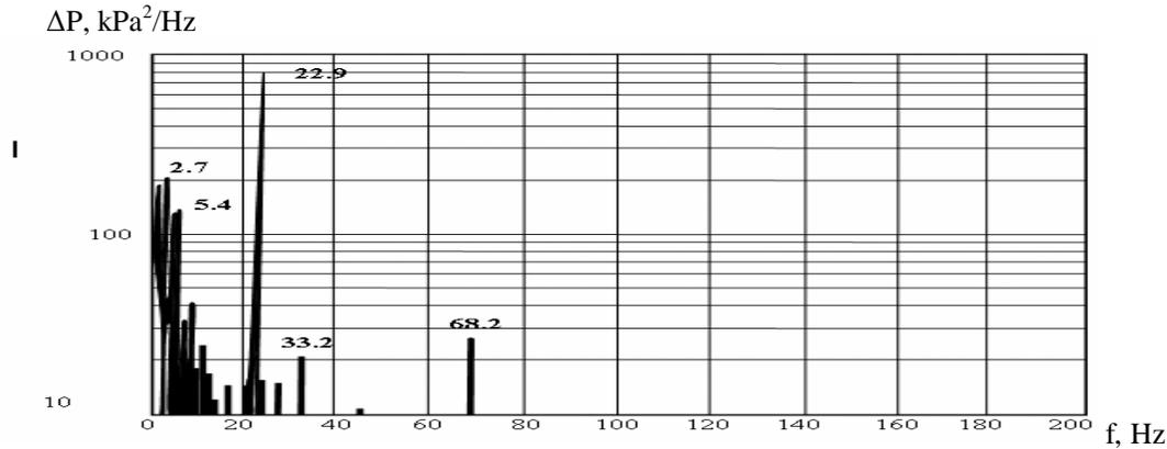
Figure 3 The APSD spectrum of pressure pulsations. TPP BP-11 (main pipelines, first loop, core outlet). For working MCP 1,2,4,  $P=16.0$  MPa,  $T_{outlet}=314$  °C,  $T_{inlet}=285$  °C.
