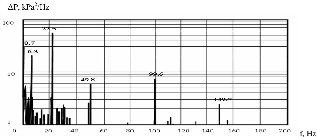
Figure 4 The APSD spectrum of pressure pulsations. TPP BP-11 (main pipelines, first loop, core outlet). For working MCP 1,2,3,4,  $P=16.0$  MPa,  $T_{outlet}=318$  °C,  $T_{inlet}=287$  °C.
