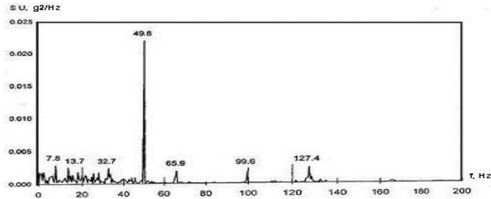
Figure 1 The spectrum of vibro acceleration. Transducer O2BI-1 (installed at top reactor unit). For working MCP 1,2,3,4,  $P=15.9$  MPa,  $T=270^{\circ}\text{C}$ .
