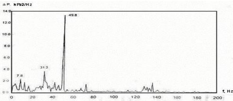
Figure 2 The spectrum of pressure pulsations from TPP BP-8 (reactor internals, reactor barrel, exit from loop No 4). For working MCP 1,2,3,4,  $P=15.9$  MPa,  $T=270^{\circ}\text{C}$ .
