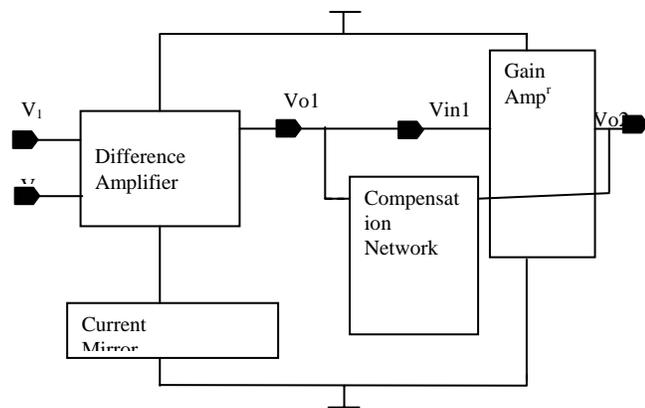
Fig. 2. Structural Partitioned Hierarchical Blocks of Op-amp
