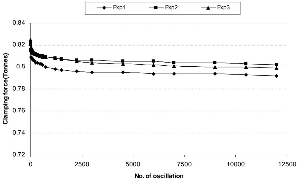
Fig. 5: Testing results for 3/8 inch BSW high tension steel bolt with outside serrated washer
