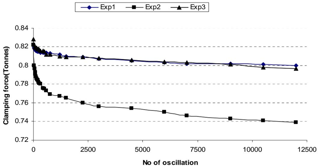
Fig. 2: Test results for 3/8 inch BSW high tension steel bolt with conventional nut
