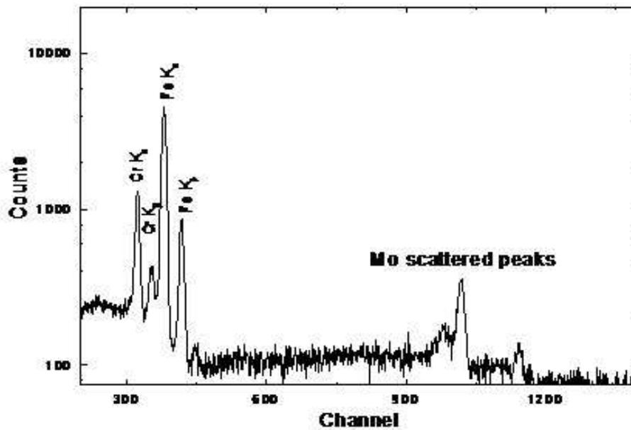
**Figure 4.** Spectrum from a Two Rupee Indian coin of 2008. Other conditions are the same as in Figure 3.
