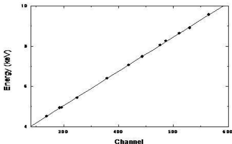
Figure 5. Energy calibration curve used in the present measurement.
