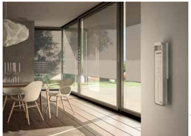
**Figure 1:** Occupant control of motorised blind using a wall-mounted controller. The controller fits in a holster on the wall, so can be removed and used as a hand-held remote
