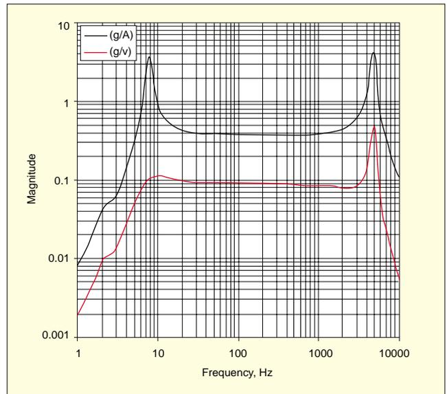
Figure 5. Transfer functions describing table acceleration per amp (upper curve) and per volt (lower curve) show the damping induced by the 'back-emf.'
