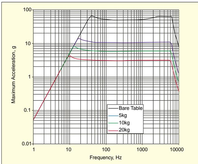
Figure 13. Effect of payload weight on maximum table acceleration with load leveling.
