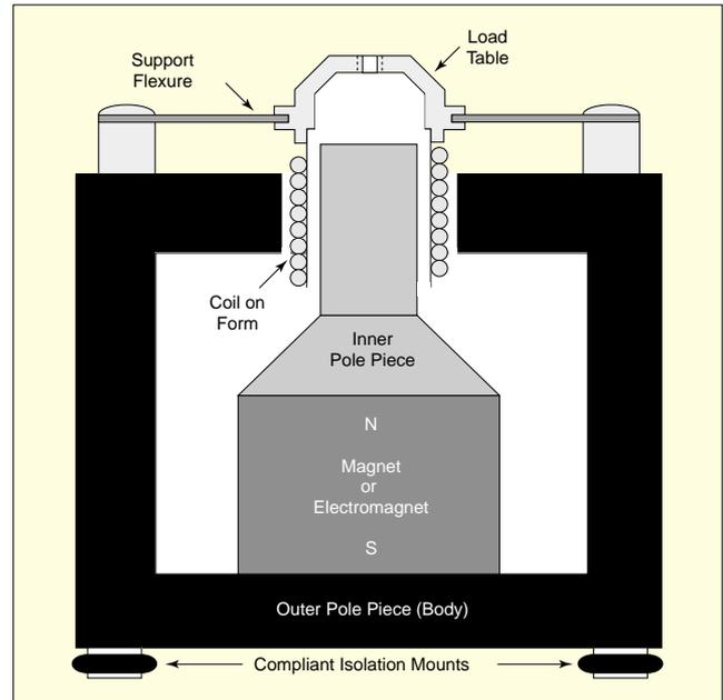
Figure 1. Soft iron pole pieces bend and concentrate almost all of the magnetic field into a very narrow gap. The armature coil is centered in this gap using support flexures (for small shakers) or rollers (for large shakers). Significant compliant connections include the support flexures, the isolation mounts and the connection between the coil and the Load Table
