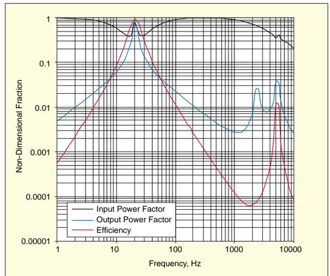
Figure 16. High Electrical Power Factor (top curve) indicates phase co-incident of voltage and current while low Mechanical Power Factor (middle curve) indicates quadrature phase between force and velocity. At most frequencies this results in less than 1% Efficiency (lower curve) for the conditions of Figure 15.
