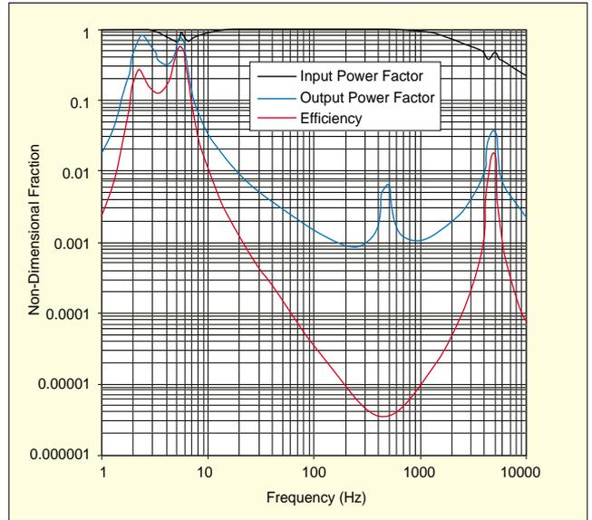
Figure 20. Efficiency and Power Factors exhibited during 25 kg shake on isolated shaker. In particular, note the improved efficiency (lowest curve) around the isolation-mode natural frequency caused by improved output power factor.
