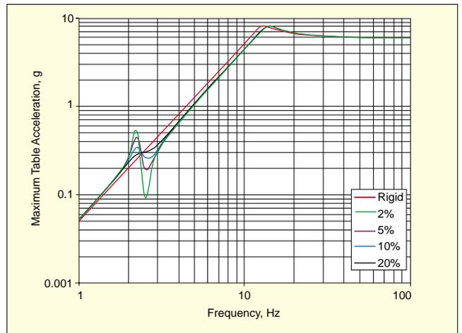
Figure 10. Effect of trunnion-base isolation damping factor on stroke loss.
