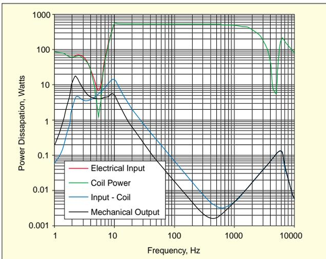
Figure 19. Repeat of 25 kg test on a shaker with trunnion base isolation (2.5 Hz, 20%). Note the mechanical output power no longer accounts for the full difference between input and coil dissipation.
