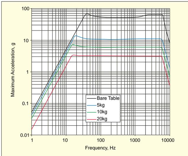
Figure 12. Effect of payload weight on maximum table acceleration without load leveling.
